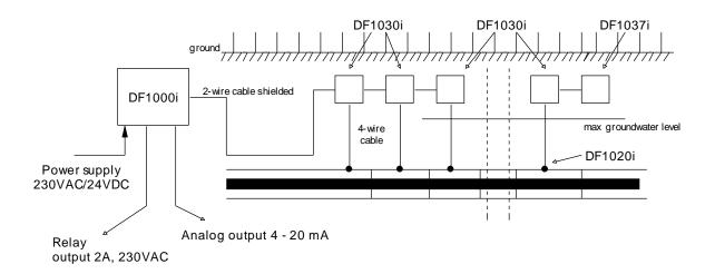
The DF1000i leakage monitoring system is an intellectual system for double pipe systems, divided in compartments.
